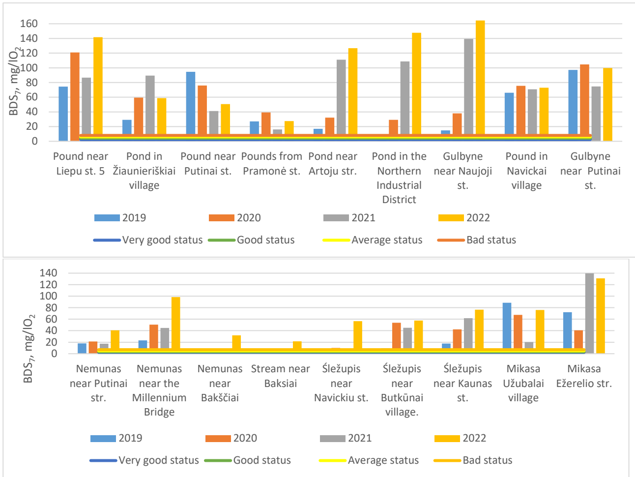
Figure 6. The biochemical oxygen demand after seven days (BOD 7 ) for pond and river water
