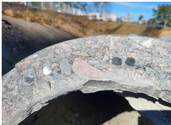
1 pav. Centrifuguotos atramos pjūvis, eksploatacija 32 metai Fig. 1. Centrifuged support cross-section, service life: 32 years
