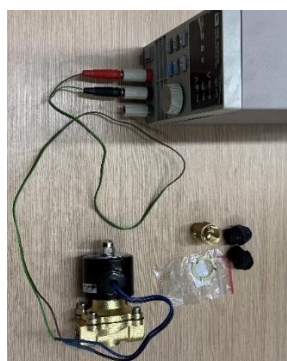
2 pav. Elektromagnetinis vožtuvas pralaidumo matavimams atlikti Fig. 2. Electromagnetic valve for throughput measurements
