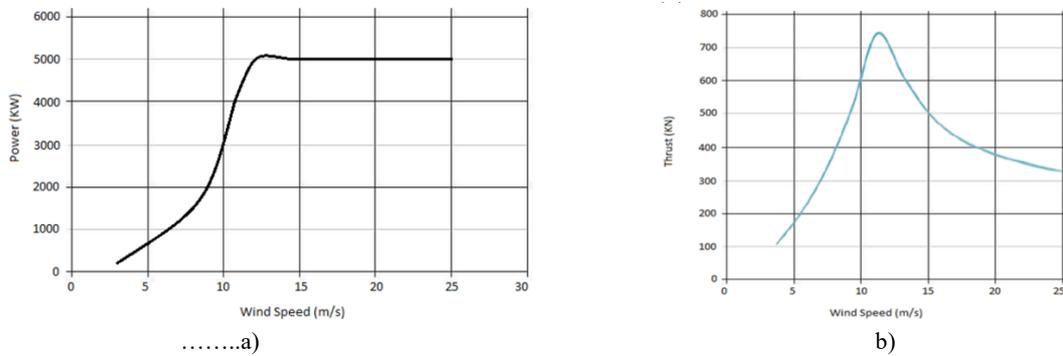
**Fig. 5.** Power & Thrust Curve
