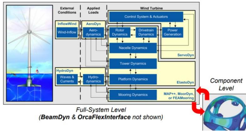
**Fig. 1.** Simulation framework for floating offshore wind turbines, showing interactions between aerodynamics, hydrodynamics, structural dynamics, and control systems.
