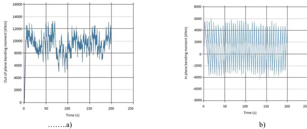
**Fig. 7.** Out of plane & In-plane bending moment (Turbulent Wind)
