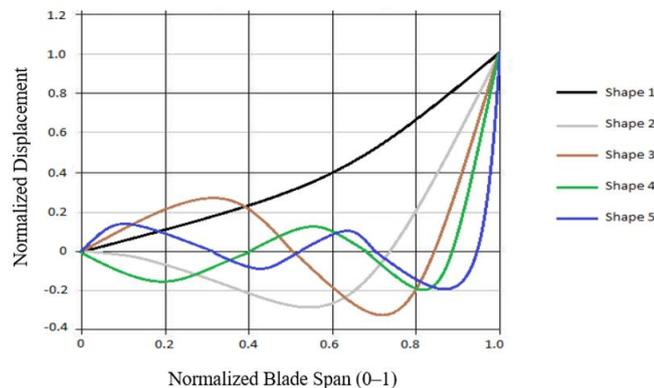
**Fig. 3.** In plane mode shapes (Blades)
