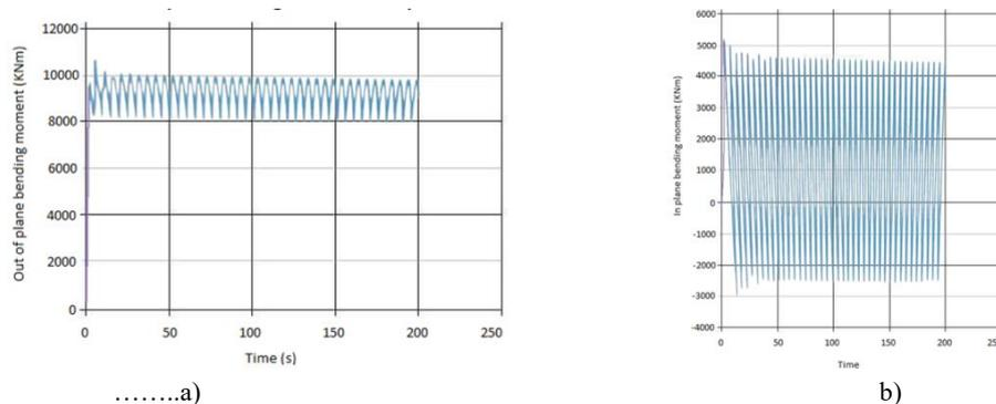
**Fig. 6.** Out of plane & In-plane bending moment (Steady Wind)
