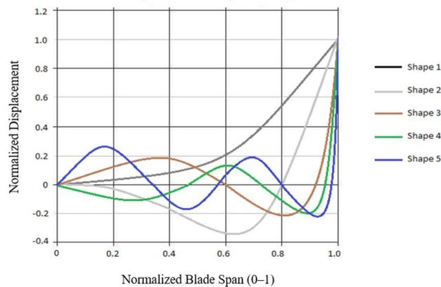
**Fig. 2.** Out-of-plane mode shapes (Blades)
