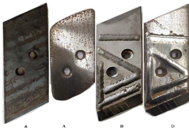
7 pav. Kaltai A ir sustiprinti kaltai D iki ir po lauko bandymo Fig.7. Plough point A and reinforced D wear before and after field experiment
