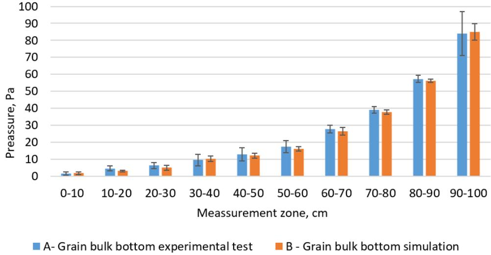
**Fig. 5.** Measurement and simulation results at the bottom of the grain bulk with a 23° repose angle under an airflow of 118 m<sup>3</sup>/h
