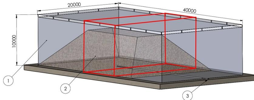
**Fig. 1.** Modeled grain storage facility and its equivalent cross-section: 1 – storage facility; 2 – grain bulk; 3 – ventilation duct.
