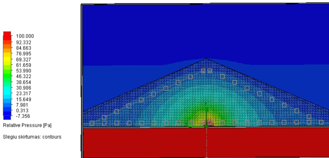
**Fig. 4.** CFD simulation of the grain bulk with a  $23^\circ$  angle of repose
