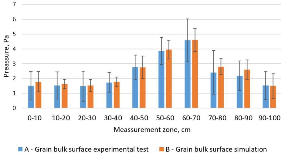
**Fig. 6.** Measurement and simulation results at the surface of the grain bulk with a 23° repose angle under an airflow of 118 m<sup>3</sup>/h
