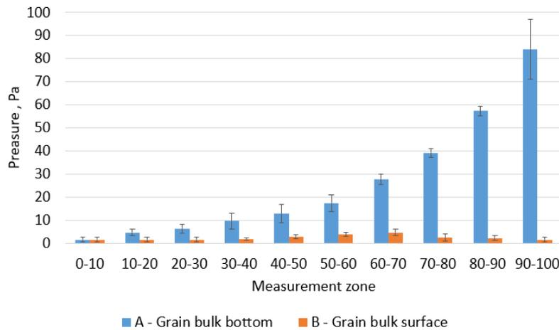
**Fig. 3.** Airflow pressure distribution in the grain bulk with a 23° repose angle
