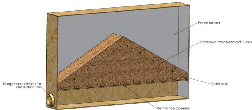
**Fig. 2.** Schematic diagram of experimental test stand
