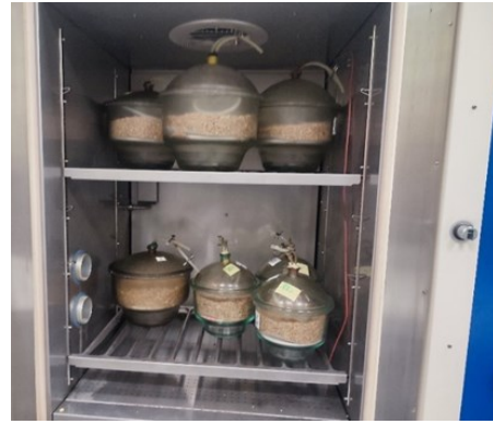
Fig. 2. Desiccators with wheat samples in a climatic chamber
