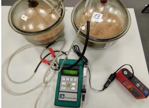
Fig. 1. Measurement of carbon dioxide (CO 2 ) concentration in desiccators with grains
