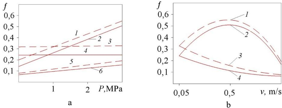
**Figure 4.** Dependence of the friction coefficient  $f$  of steel 37Cr4 in an acidic environment on pressure  $P$  (a) and the sliding speed  $v$  (b); dashed lines – without hardening; solid – after nitriding (a: 1, 2 –  $v = 0.15$  m/s, 3, 4 – 0.05, 5, 6 – 1; b: 1, 2 –  $P = 4$  MPa, 3, 4 – 1).
