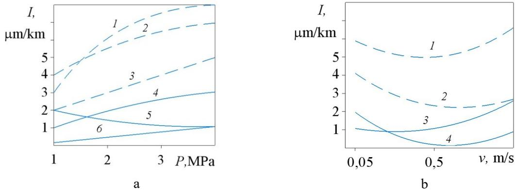
**Figure 3.** Dependence of the wear intensity  $I$  of steel 41CrAlMo7 in an acidic environment on pressure  $P$  (a) and sliding speed  $v$  (b): dashed lines – without hardening; solid – after nitriding (a: 1, 4 –  $v = 1$  m/s, 2, 5 – 0.05, 3, 6 – 0.5; b: 1, 3 –  $P = 4$  MPa, 2, 4 – 1).
