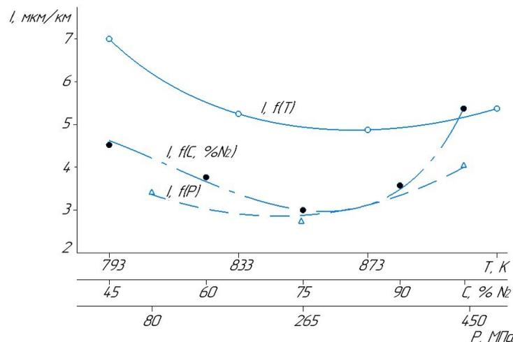
**Figure 6.** Dependence of the intensity of wear  $I$  of steel 37Cr4 in an acidic environment on the parameters of ionic nitriding (wear test mode: sliding speed  $v = 1$  m/s, pressure  $P = 4$  MPa): 1-  $I=f(T)$ ; 2-  $I=f(C, \% N_2)$ ; 3-  $I=f(P)$ .
