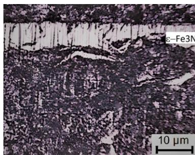
**Figure 2.** Microplates of nitrided steel 37Cr4 (8.7μm – nitride zone; 300μm – modified zone).
