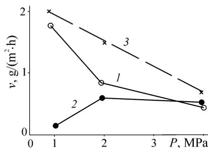
**Figure 5.** Dependence of the corrosion rate (curve 1), mechanical (2) and total (3) wear during friction of steel 40X in an acidic environment on the pressure is the friction contact  $P$  ( $v = 0.05$  m/s).
