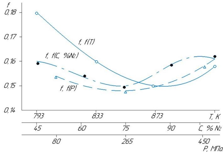
**Figure 7.** Dependence of friction coefficient of steel 37Cr4 in an acidic environment on the parameters of ionic nitriding (wear test mode: sliding speed  $v = 1\text{ m/s}$ , pressure  $P = 4\text{ MPa}$ ): 1-  $I=f(T)$ ; 2-  $I=f(C, \% N_2)$ ; 3-  $I=f(P)$ .
