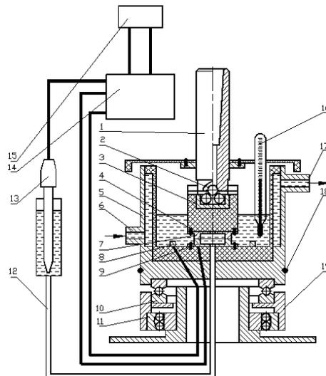
**Figure 1.** Installation of end friction: cone 1, four balls 2, body 3, screws 4, electrochemical cell 5, upper sample 7, fitting 6-17, electrode 8, lower sample 9, bearings 10-11, tube 12, reference electrode 13, potentiometer 14, potentiometer 15, thermometer 16, housing 18.
