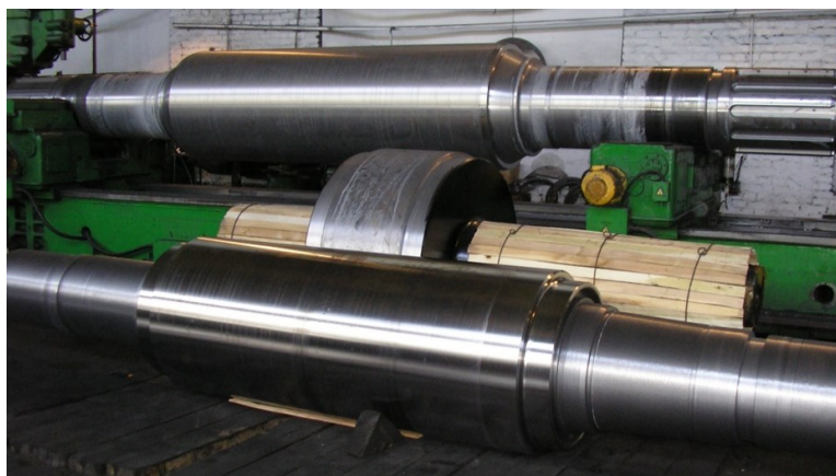
Figure 1. Centrifugal cast rolls with a working layer of chromium cast iron.
