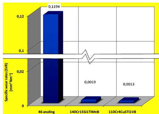
**Figure 3.** Two-body abrasive wear of hardfacings.
