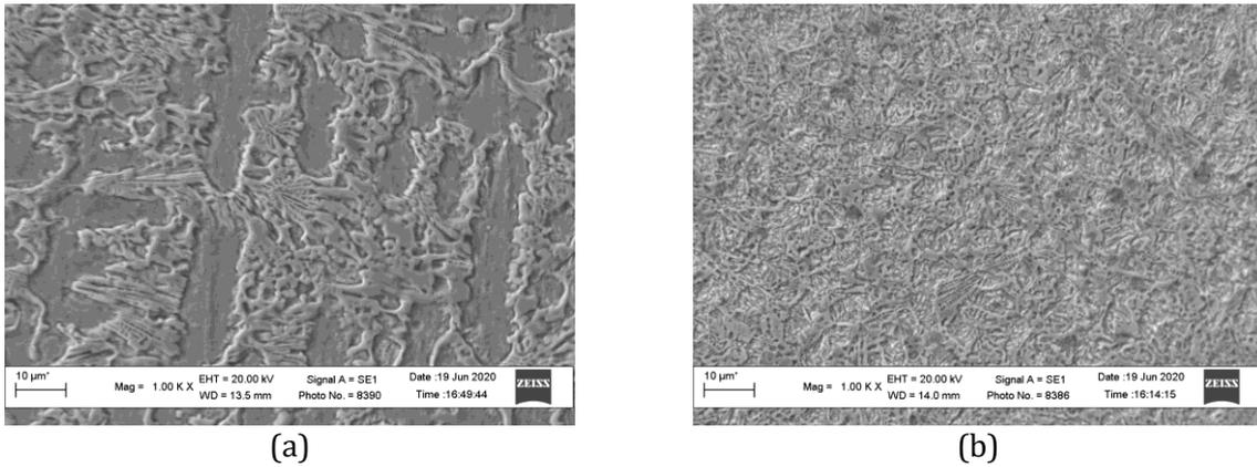
**Figure 2.** SEM images of the microstructures  $\times 1000$  (a) deposited metal hardfacing by: (a) FCAW-S-140Cr15TiSi1MnVB and (b) FCAW-S-110Cr4Cu5Ti1VB with exothermic addition (CuO–Al).
