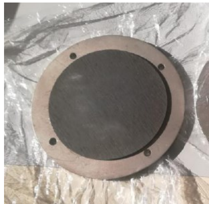
Figure 1. Sample material added to the rotating disk of the test apparatus.
